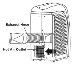
The hot exhaust air can be vented through the wall or out a window. If mounting in the wall, the height of the hole should be  $14 \ 1/4"$  to  $60 \ 5/8"$  (36cm to 150cm).
